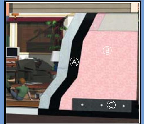
TUFF-N-DRI offers a reliable system to control moisture, including water under hydrostatic pressure:
