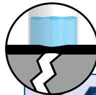
Membrane elongates to span a shrinkage crack, and effectively resists hydrostatic pressure.
